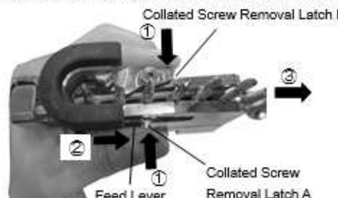
① Hold the attachment on one hand meanwhile pressing onto the collated screw removal latch A & B.
