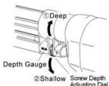
① Turn the screw depth adjusting dial upward to achieve more depth.
