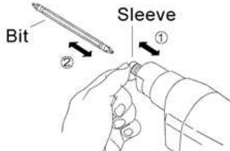
**Attaching** ①Pull and hold sleeve toward the electric driver.
