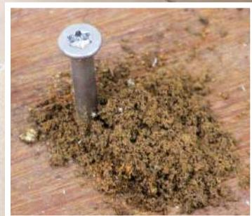
The unique drill tip bores a pilot hole while threading itself into the wood ejecting sawdust in the process
